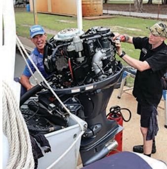
Graham and Caleb from Northside Marine performing the service on Jonkers Bribie 3's Yamaha 130HP outboard.
