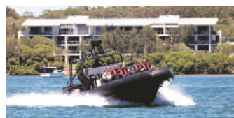
QPV Tactical Response Vessel Casey Blain, equipped with 3 x 350hp V8 out-board motors, capable of in excess of 50 knots. Above: Casey Blain, in action and some smiling faces after a short trip.
