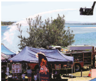
The water cannon from QFES's appliance 511 India sprays some water around from the unmanned aerial platform. This appliance is capable of extending the platform to 42m to rescue victims or fight the fire with the water cannon, capable of discharging 4,500 litres per minute onto the fire.
