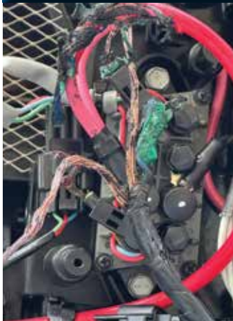
Port engine on B2 won't trim/tilt, wires & electronics that control this got fried.
