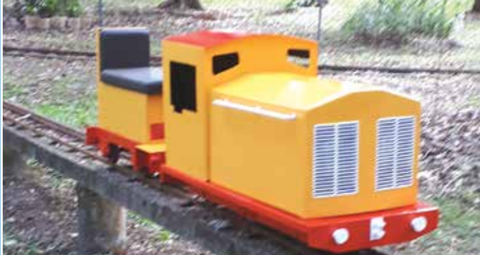
Neverfail is a 7 1/4" 24-volt loco, which, as its name implies, never stops pulling passengers.
